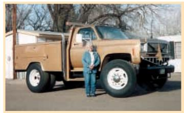
Bill Swets cut the cab and utility bed off his Chevy 3/4-ton pickup and mounted them on the frame and running gear of a school bus. Big pickup stands  $7\,\mathrm{ft}$ .  $10\,\mathrm{in}$ . tall.
