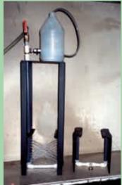
Powered "boot wash" is fitted with 16 water jets - 8 on each side. It runs off a garden hose. To clean your boots, you simply stick them one at a time into the jets. Large unit for hog producers (left) dispenses disinfectant with the water. Disinfectant is sucked out of a 1-gal. jug that sets on top of unit.
