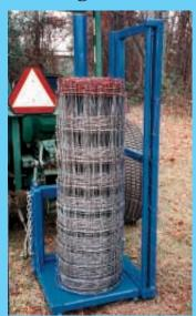
Fence Caddy allows one person to install fencing using a tractor. It picks up the roll, unrolls the wire, and stretches it. Fencing is fed out through a locking device that pulls it taut while you fasten it to your nosts.
