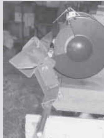
Sharpener is designed to fit onto any 6 or 8-in. bench grinder.
