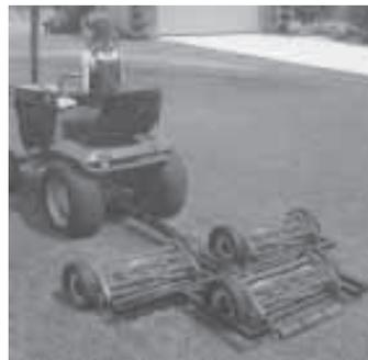
Reel mower can be pulled by any lawn tractor or ATV.
