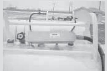
Porter Bros. device fits over valves on ammonia tank and then locks. It's made from stainless steel.
