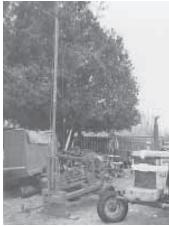
To make the well-drilling rig, Kendall mounted a 15-ft. tall derrick on an axle, along with a 14 hp gas engine.
