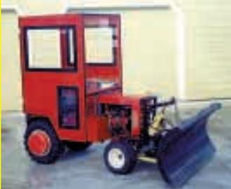
in. thick plywood doors and big windows on all sides so the driver has a great view. The windows are acrylic plastic panels which are much safer than glass and won't shatter. The windows are screwed into wooden frames from the outside so they can be easily removed if they ever crack or break. The cab doesn't have a heater, but the windows are big enough that sunlight helps heat up the cab during winter.
