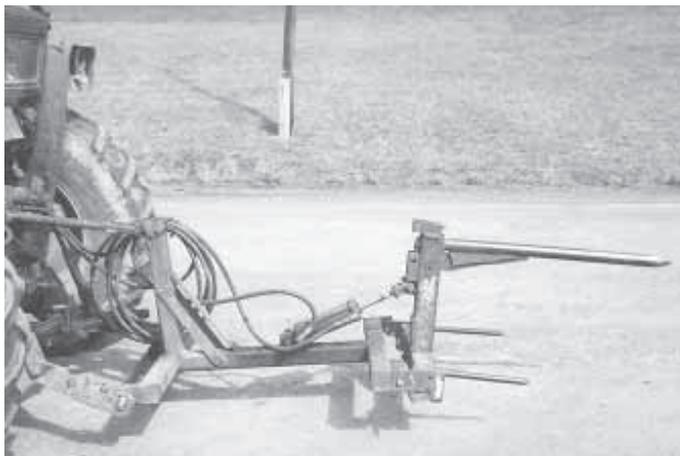
Home-built, 3-pt. mounted bale handler lets Clark stack bales onto a pickup.
