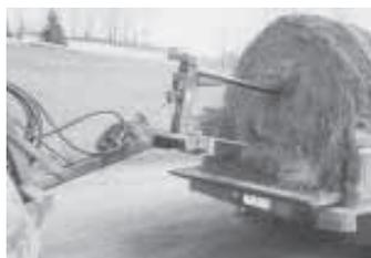
Frame is made from 3 1/2-in. heavy-walled sq. tubing. The single spear was made from a 2 1/2-in. round bar.
