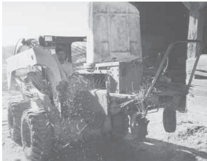
Brian Cope modified a chopper that originally mounted on a 4-wheel handcart and mounted it on front of his skid loader. Chopper is powered off loader's hydraulics.
