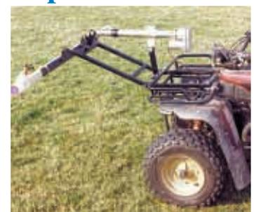
Optional electric lift operates off ATV battery.
