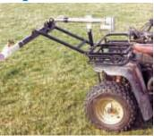
Optional electric lift operates off ATV battery.
