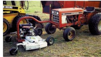
The 60-in. AcrEase mower deck mounts on front of Reynolds's Lo Boy tractor. Gooseneck ball hitch allows mower to swivel 360 degrees when turning or backing up.
