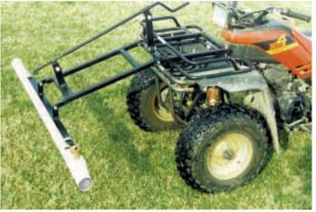
Kit turns any ATV into a self-propelled weed wiper. Crank shown above is operated manually and lets you raise or lower height of wiper on-the-go right from the seat.
