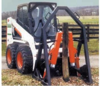
Post puller uses a pair of angled "tooth bars" to bite into post before pulling it out of the ground.
