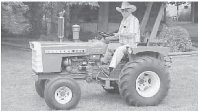
Beneath this "half-scale" Oliver tractor is the frame of a Yanmar 1510 tractor, which was rebuilt to Oliver "specs".
