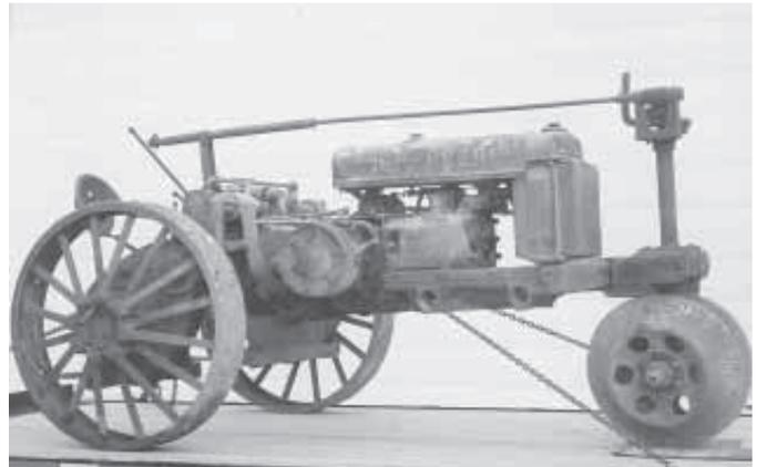
Experimental 1929 Deere GP has modified rack-and-pinion power-adjustable rear axle and over-the-top shaft steering. It was identified by a distinctive dent.
