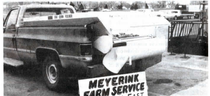
Steel box fits into pickup bed, and apron chain drops feed into rear-mounted auger.
