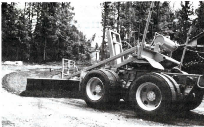
Grader blade attaches to fifth wheel and is operated by air power.
