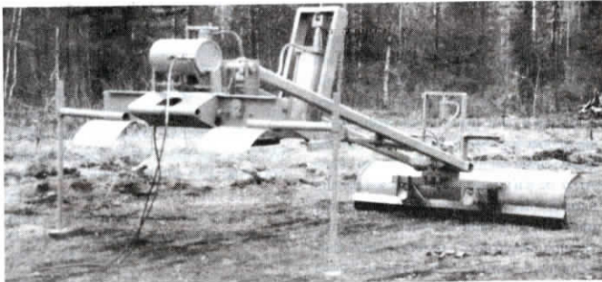
Toggle switches mount on control box attached to cord that runs from cab to blade.
