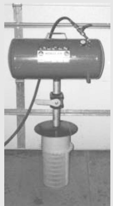
**To clean a filter, Miller places it on the shop floor and sets the tank on top of it with a sheet metal circle over the filter. He then opens a valve to release air pressure.**
