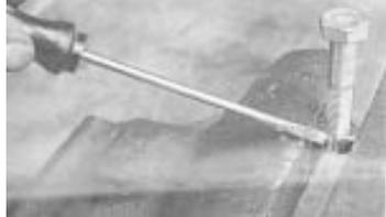
out of the side of a nut, and then screw the nut onto the bolt and clamp it into the vise. The nut will clamp down on the threads without damaging them, holding tightly. When the vise is released, the nut will screw right off.
