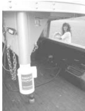
Self-guiding, self-latching coupler attaches to trailer hitch and guides ball into locking position anywhere within a 6-in. "capture" area.
