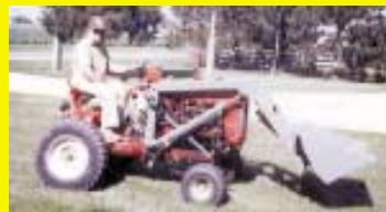
made the front axle from trailer parts that I already had. The tractor rides on 7.50 by 16 rear tires. The front tires, which are smaller, are off an old riding mower.
