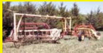
the hitch and mounted it on an old wagon running gear. I use a hydraulic cylinder to move the rear rake in or out in order to control the windrow width. A swivel mechanism allows the axle to tilt up or down over bumps. (Matt Fordyce, 413 Peterson, Alta, Iowa 51002 ph 712 284-1052; E-mail: g.miller@ncn.net.)
