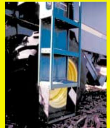
I added extra railings and step extensions to my Deere tractor and combine as shown above in the photos. Makes it a lot easier to get on and off. (Byron Rhodes, 14870 US Hwy 65, Zearing, Iowa 50278 ph 641 487-7365)
