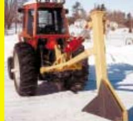
with an interesting new use. I made them a special 3-in. boot with a 6-in. flat front which pulls 30 percent easier. Owners in Kansas and Utah are using the 3-in. boot to lay 1 1/2-in. schedule 40 plastic conduit for electrical lines for irrigation. Another individual is buying one for a vineyard to run 3-in. tile between his grape vines. One more is buying one to run 1 1/2-in. water line on his ranch in Wyoming.
