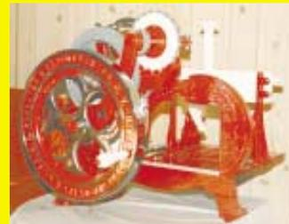
flywheel and other parts. There's no stainless steel in this slicer. Just a lot of cast iron and steel. It has a sliding table which slides at the turn of the wheel. It'll do everything from shaving thin slices to cutting big chunks.
