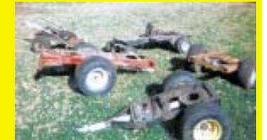
just build a cargo box out of plywood to fit on top, and make a tow bar. Works great to pull behind a newer garden tractor.
