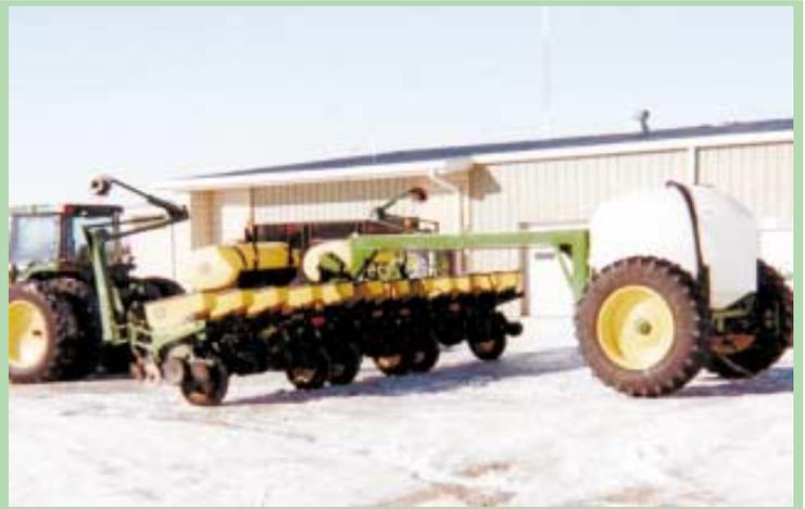
Cart is designed to hold a 1,400-gal. cone-bottom tank, which Ensz says has a low center of gravity and keeps sloshing to a minimum.
