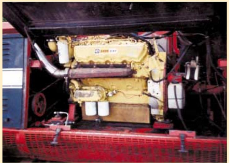
Pat Minehan found out that repairing or replacing the 540 Perkins diesel engine in his Massey Ferguson combine would have been too expensive. He decided to "upgrade" to a Caterpillar 3208 diesel that came out of a New Holland TR70 combine..
