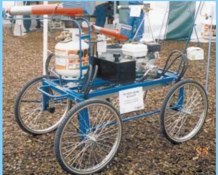
"Robot" scarecrow consists of a hydraulically-driven cart fitted with four narrow bicycle-type wheels. A cannon and tank mount on bed of cart.
