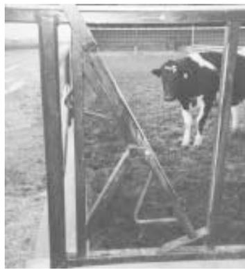
A steel bar pivots at the middle and can be moved to either side of a pin (at top).
