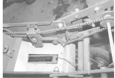
"Shield" bolts below bottom of seed box to help prevent dirt and corn stalks from getting into seed metering chains and sprockets.
