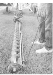
A length of rebar attached to back side of sweep serves as a handle, allowing Gass to pull auger from a safe distance.
