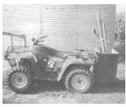
"It works better than the ATV's original factory-made racks for carrying both long and short objects," says Chad Wernimont, about the wooden box he mounted on back of his ATV.
