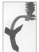
"Trash Boards" consist of a pair of wings with a steel strap at bottom that bolts to chisel plow's shank.
