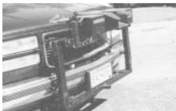
Fifth wheel hitch bolts to top of a rectangular frame that bolts to pickup chassis.
