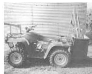
"It works better than the ATV's original factory-made racks for carrying both long and short objects," says Chad Wernimont, about the wooden box he mounted on back of his ATV.
