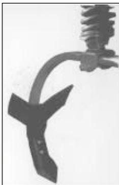
"Trash Boards" consist of a pair of wings with a steel strap at bottom that bolts to chisel plow's shank.
