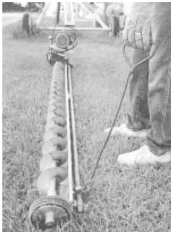
A length of rebar attached to back side of sweep serves as a handle, allowing Gass to pull auger from a safe distance.
