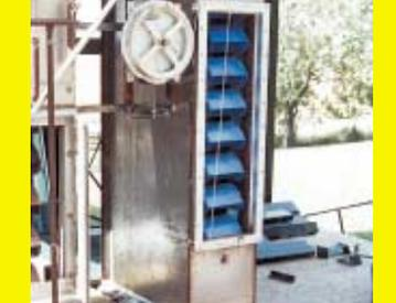
in. high by 10 in. wide. We bought them from a local company that sells components for grain legs and fertilizer plants, etc. The plastic buckets are corrosion resistant and are usually used by fertilizer companies. They were priced comparable to steel buckets. The only problem is that if they get bent you can't beat them back into shape like steel ones. We also bought a new set of belts to support the buckets. **(Clair Wilson, 132 Hillview Rd., Winchester, Ill. 62694 ph 217 742-3809 or 3918)**
