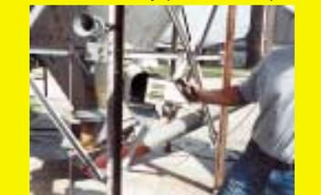
grain moisture tester. Grain is delivered from a dryer into the bin. It's unloaded out an auger at the bottom of the bin and into a grain cleaner. From there it's pneumatically delivered into a 10,000-bu. bin. I use the tester to check grain moisture every time a new load of grain is loaded into the bin. Not only is the tester always within easy reach but it's out of the weather, too.
