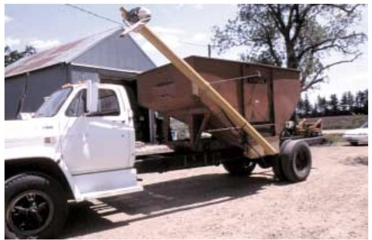
An orbit motor at top of auger plugs into outlets on tractor that Reed uses to pull his grain drill.
