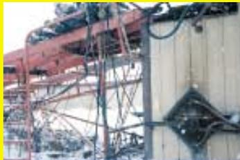
Ramp drops logs into furnace. Note ash cleanout door on end of furnace.
