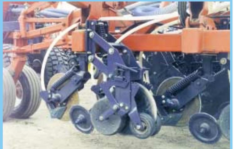
**Hermans' opener makes use of wheels on either side of opener to hold crop residue in place while a single disc slices through it, opening up a clean seed slot.**
