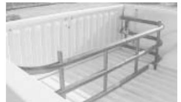
Unit flips forward when not needed, providing a 2-ft. wide enclosed area behind tailgate where you can contain small loads.
