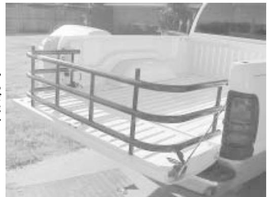
"Bed X-Tender" adds 2 ft. of cargo space to bed of pickup by closing in the tailgate.
