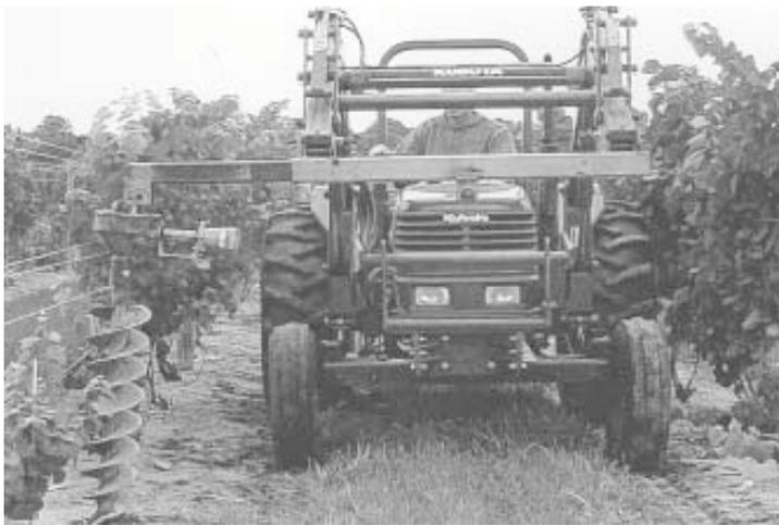
Auger attaches to end of a telescoping tube that mounts on Thompson's front-end loader. Telescoping tube is operated by the tilt function on tractor's loader control.
