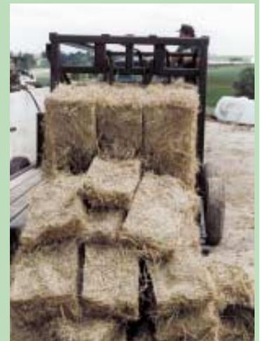
Bale slicer consists of a box frame with a ram or plunger at one end and knives at the other. Bale is pushed back through knives by plunger.
