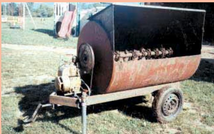
Spreader was made from a 250-gal. fuel tank. To create the flail bar, Martin welded chains to opposite sides of a steel pipe at 5-in. intervals.
