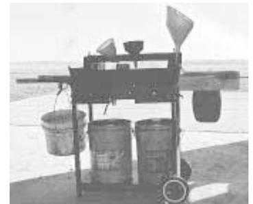
"It works great for draining the oil from our Steiger tractors. The grill is only 3 1/2 ft. high so I can wheel it right under the tractor," says Sproule.
