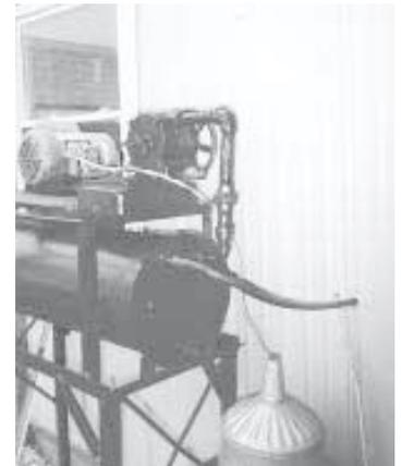
Suction hose from tank runs through hole in shop wall.
