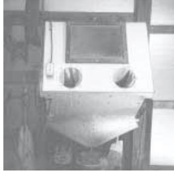
Graham built his sand blasting cabinet out of a top-loading washing machine. Hand holes and a large window install on front side.
