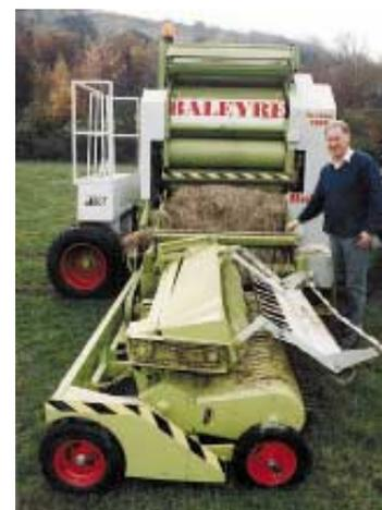
Baler's double wide bale chamber runs at right angles to direction of travel. There's no need to wait for bales to be wrapped.
