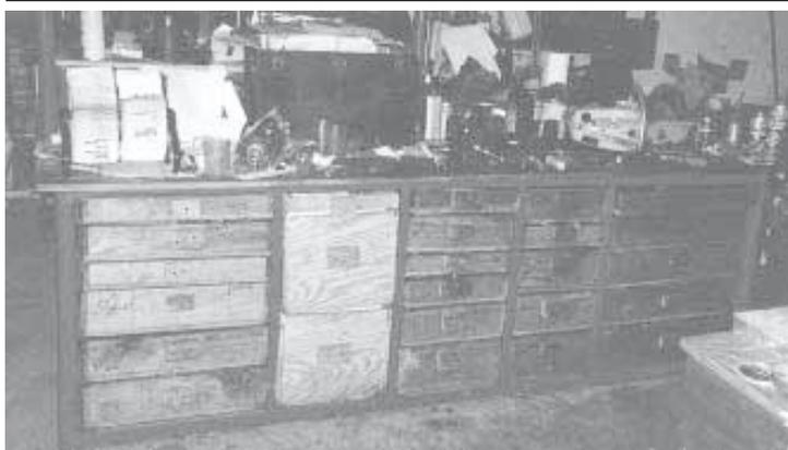
**John Aaron Rissler, New Enterprise, Pa.:** "Needing both a tool chest and a work bench, I decided to combine both by building what I call a Tool Bench. I needed all sizes of drawers - wide and narrow, deep and shallow. I used sq. steel tubing to make the frame and angle iron to make the drawer slides. I didn't really count the drawers but just figured the different sizes I wanted.
