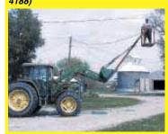
I thought your readers would like to see the basket lift we made for our loader tractors. The basket has a 25-ft. reach and is free-swinging so it always stays in the upright position. The boom that holds the basket bolts onto the bucket floor with four bolts and is chained to hooks welded on top of the bucket.
