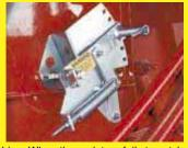
bine. When the rock trap fails to catch a rock, it goes through the cylinder and other threshing mechanisms and into the stubble chopper. The chopper has a rotating drum with rigid or swinging hammers attached to it. The flail hammers pass through a multiple arrangement of U-shaped brackets (or Clever-Tech's sickle section choppers) which are rigidly attached to the chopper bar. Normally, it is U-shaped brackets – or sickle sections - that break.
