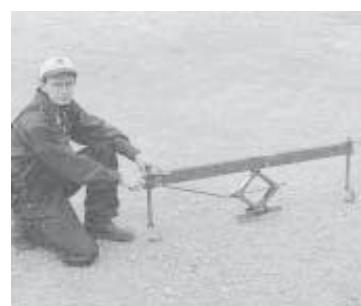
Automotive screw jack mounts at center of 5-ft. length of 2 by 3-in. steel tubing, the outer arms. Now, with the 12-in. throat, the screw jack is past half-way before it starts to push on the chain slat.
