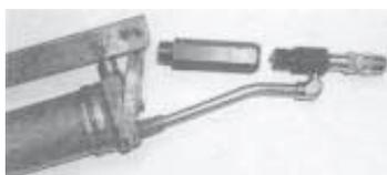
**Grease gun screws onto elbow fitting on side of unit.**
