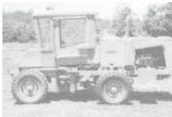
**This 4-WD articulated tractor is powered by a V-6 engine and transmission out of a Chevy S-10 pickup.**
