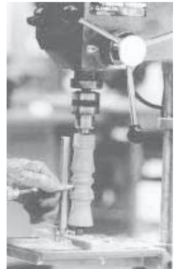
Vertilathe can be used to work on pieces up to 3 in. dia. Comes with two stainless steel tool rests.
