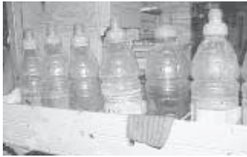
Dulas uses plastic squeeze bottles to hold cutting oil and other liquids.
