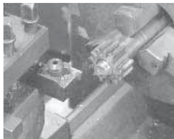
MacGuire resplined the steering gear from his Case 195 on his benchtop mill.
