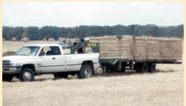
"Hay Hawg" is fitted with its own power unit which provides hydraulics and electronic controls. Rig will pick up and transport 10 round bales behind a 3/4-ton pickup.
