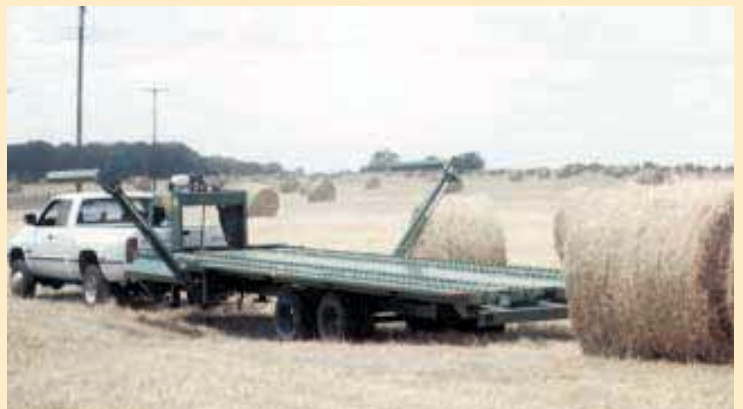
Lift arms on either side of trailer load bales onto deck where chains move them backward.
