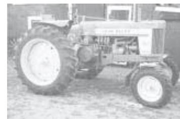
Fisher uses his Deere 720 diesel to pull a 16 1/2-ft. disk and a 4-bottom plow.
