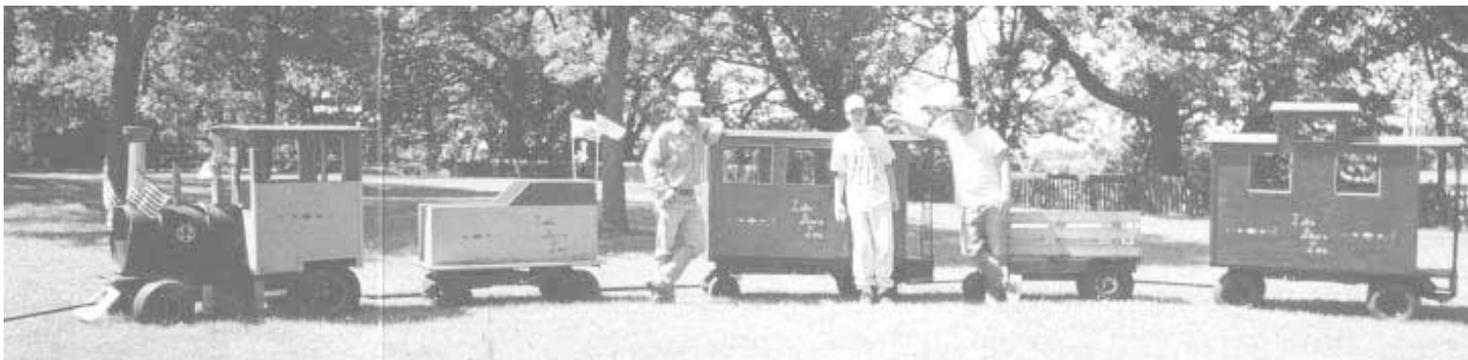
The 35-ft. long, five-unit train hitches behind Thompson's Deere 112 garden tractor. It includes a steam locomotive, coal tender, passenger car, cattle car, and caboose.
