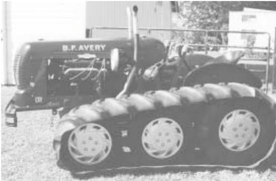
**Full Track** - This 1946 Avery rides on a pair of 18-in. wide, 38-in. long rubber tracks made from two rear tractor tires off a Deere 4340 tractor. The tracks are supported by three sets of axles. The center and front axles are rear axles off Oldsmobile Cutlass front wheel drive cars. The rear axle is original
