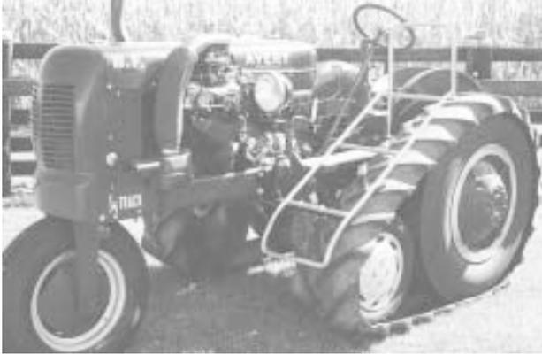
**Half Track** - This 1946 Avery is equipped with 15-in. wide, 38-in. long "half tracks" and a single 16-in. front wheel. The track was made by cutting up tractor tires. It's powered by a V-6 turbocharged engine off a Buick Regal car and also has the car's automatic transmission. The track is supported by 22-in. tires on back and 14-in. tires up front. The axle that connects the front tires pivots to
