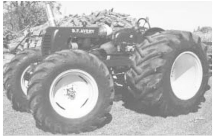
**4-WD "Big Foot"** - "Everyone wants to see me drive this one," says Melton. It's a 1946 Avery equipped with a Jeep front axle and four huge combine tires - 30.5 by 32's on back and 14.9 by 26's on front. A 4-cyl. Hercules turbocharged engine supplies the power and is connected to the tractor's
