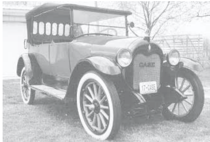
Ellis occasionally displays his restored "Case" cars at old-time machinery shows. This one is a 1917 40 hp "T" 7-passenger model.
