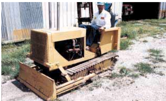
Moss's "mini dozer" started out as an old David Bradley SP trencher.
