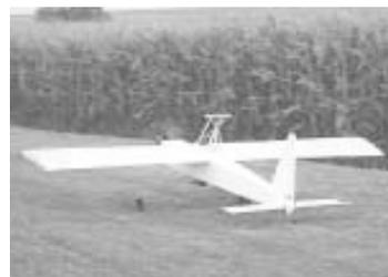
Wood-framed plane has a 10-ft. wingspan and is powered by a 2-cycle gas engine. Plane is fitted with a bomb bay and radio-controlled door as well as radio-fired "air-to-air missiles".
