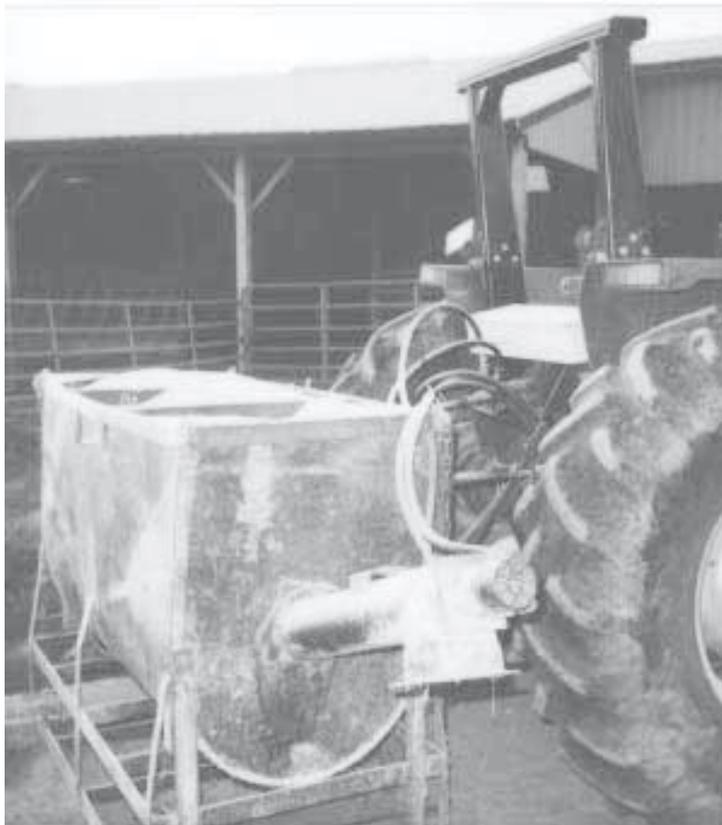
Barrel is open on top. A hydraulic-powered auger mounts on one side.
