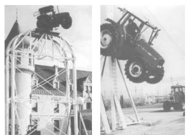
Rupert Ebner drove a tractor up and over this 39-ft. tall metal archway. Metal plate on 3-pt. hitch runs on rollers under track.
