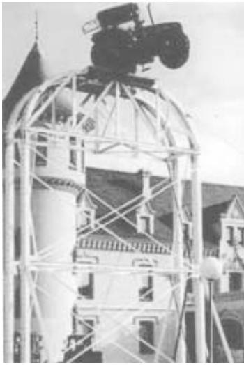
Rupert Ebner drove a tractor up and over this 39-ft. tall metal archway. Metal plate on 3-pt. hitch runs on rollers under track.
