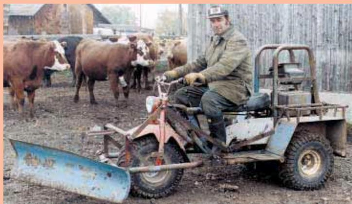
**Capiuk used steel tubing from an old combine to build the frame and fitted it with the front end off an old Honda 3-wheeler.**
