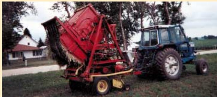
Agropack bale chamber swings back and forth, packing hay in accordion-like folds. Bales are rounded on one end to shed rain and snow.
