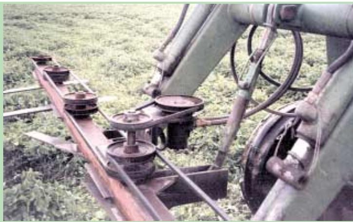
A single hydraulic motor positioned between loader arms drives all 7 blades at once.
