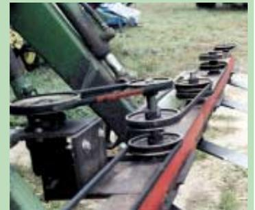
Blades mount on vertical shafts that extend through toolbar.
