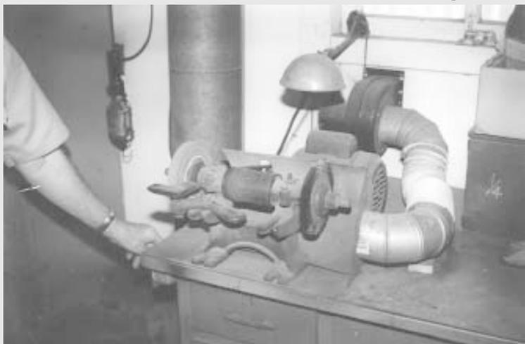
**Richard Cox, Jacksonville, Ill.:** "Grinding jobs are a lot cleaner ever since I installed a vacuum system to carry dust and small grindings out through my shop wall. I used a
