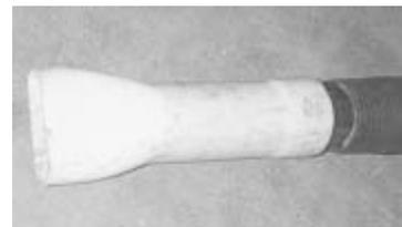
gun to heat one end of a 1-ft. length of tubing until it started to get soft, and then squeezed it between two boards to flatten it out, leaving a narrow opening. Then I heated the other end of the pipe and inserted the vacuum hose. When the pipe cooled off, I had a tight fit. I also use it to clean out grain from under the aeration floor in my grain bin. You could make the pipe as long as you need."
