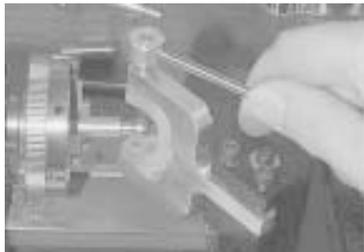
shapes or curves into brass, aluminum, steel, or plastic. The tool cuts convex curves up to 3/4 in. in diameter. Works great for making round ball joints, governor weights, railing knobs, round contact points for tools, nose cones, and many other useful and decorative objects.
