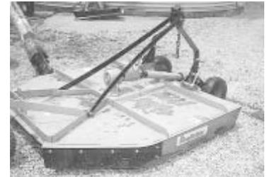
of flexible 1/2-in. thick rubber. The original metal guards would at times drag in the ground and tear it up, whereas the flexible rear shield can yield to obstacles without getting twisted out of shape. I simply bolted the rubber onto the deck."
