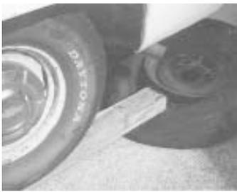
**Bill Reeks, Cromwell, Ky.:** "To break the bead of stubborn tires from the wheel rim, I lay a 3 by 4-in. board on the tire with the end close to the wheel rim and drive one wheel of a vehicle up on the board. The weight of my Suburban pops the bead loose easily. It's simple, cheap and effective."
