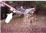
Arrow points to small electric motor that shakes tines on fork.
